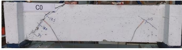
(a) Experimental crack pattern for C0
